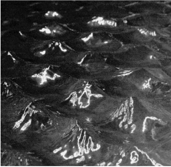
Fig. 4.30 Pyramidal waves observed by Kimmoun et al. (1999) in a laboratory tank
